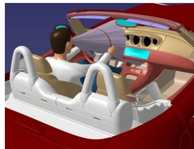
Fig. 1: Analysis of direct vision: view of the switch obscured by the steering wheel rim
