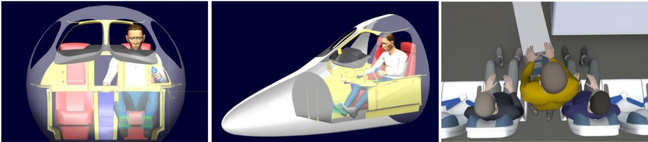
Figs. 1-3: Cockpit and passenger area layout: visibility, reachability, seating and space requirements
